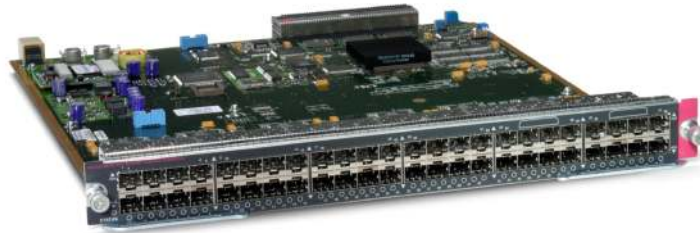
Figure 1. Classic 48 Port 100BASE-X Fiber Interface Module (part number WS-X6148-FE-SFP)
