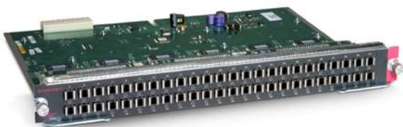
Figure 8. WS-X4148-FE-BD-LC Cisco Catalyst 4500 Series 48-port 100BASE-BX10-D Fast Ethernet Line Card for single strand of SMF
