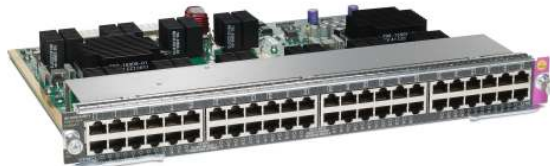
Figure 2. WS-X4648-RJ45V-E Cisco Catalyst 4500 E-Series 48-Port 802.3af PoE 10/100/1000 (RJ-45)
