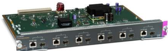
Figure 19. WS-X4506-GB-T Cisco Catalyst 4500 6-port 10/100/1000 RJ-45 PoE IEEE 802.3af and 1000BASE-X (SFP)
