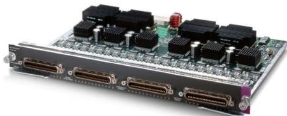
Figure 14. WS-X4248-RJ21V Cisco Catalyst 4500 PoE IEEE 802.3af 10/100, 48 ports (RJ-21)
