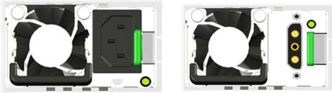
Figure 15. AC and DC Power Supplies – Connector View
