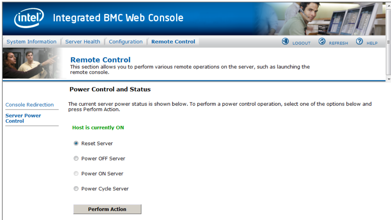
Figure 87: Remote Control Server Power Control Page on S1200BTL platforms
