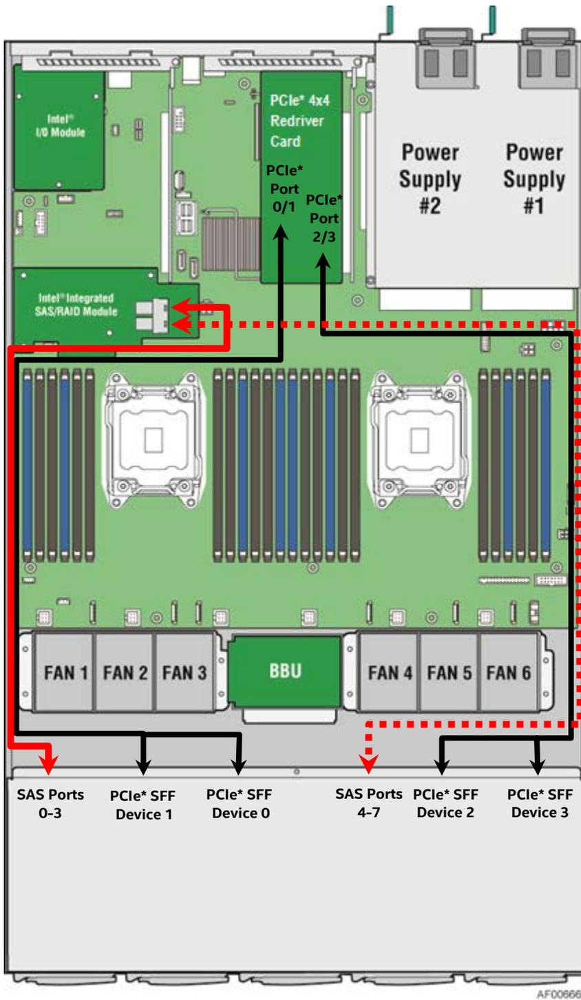
Figure 40. Combo Backplane Cable Routing – PCIe\* SFF + SAS
