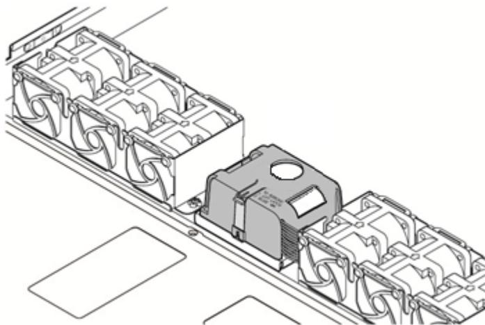
**Figure 52. Support for dual Intel® RAID Maintenance Free Backup Units (Optional Accessory)**
