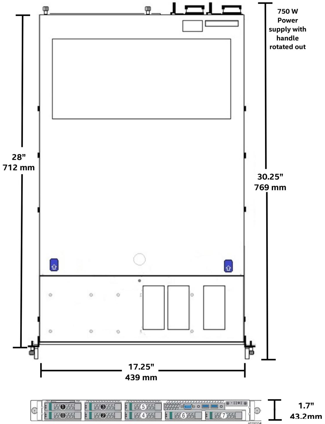
Figure 16. Chassis Dimensions
