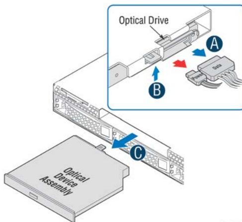
**Figure 35. Optical Drive Installation**
