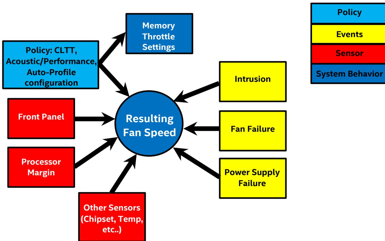
Figure 26. Fan Control Model
