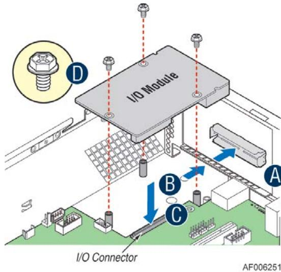
Figure 58. Intel® I/O Module Placement
