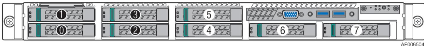
Figure 10. 2.5" Drive Bay – 8 Drive Configuration (Model R1208WTxxxx)
