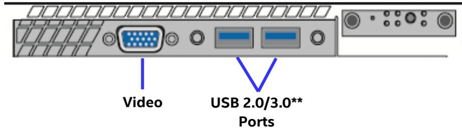
Figure 53. Front I/O Panel Features
