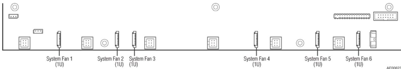
**Figure 28. System Fan Connector Locations on Server Board**
