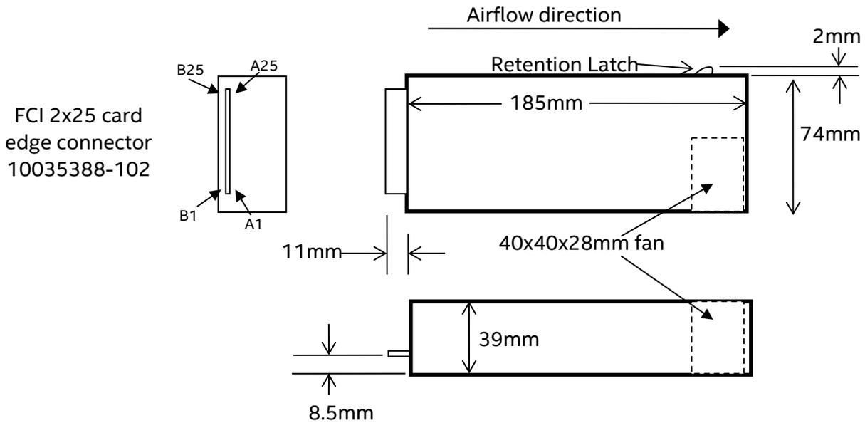
Figure 22. 750W AC Power Supply Module Mechanical Drawing
