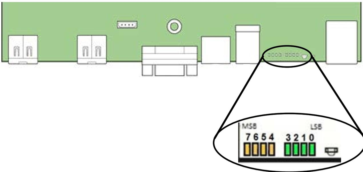
Figure 60. POST Diagnostic LED Location
