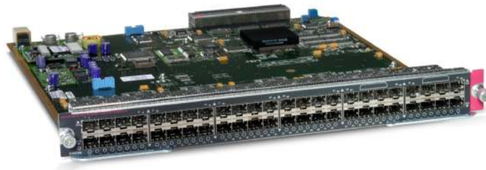
Figure 2. Classic 24 Port 100BASE-FX Fiber Interface Module (part number WS-X6324-100FX-MM)
