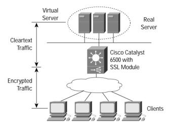
The Cisco Catalyst 6500 uses ACLs containing entries that associate IP addresses and port numbers to direct traffic flows from clients to SSL modules and from servers to SSL modules. In the client-to-server direction, the ACL identifies data flows that need to be directed to server port 443, the SSL port. The Cisco Catalyst 6500 allows normal data traffic that is not associated with an ACL entry to go directly to a server, without first directing it to the SSL module.
