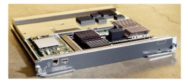
The SSL Service Module offloads all SSL processing, allowing the end Web and eCommerce servers to process more requests for content and handle more e-transactions—providing a multifold increase in the performance of eCommerce and secure sites using encryption.
