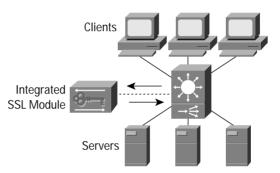
The Clients send encrypted traffic on port 443, the standard SSL port. The CSM listens on port 443 and load balances the encrypted traffic to an internal "server farm" of SSL modules. The selected SSL Service Module decrypts the traffic, stamps it with a SSL Session ID, opens a clear-text connection to a Versatile Interface Processor (VIP) on the CSM, and sends the traffic to a port that has been configured to receive "decrypted SSL traffic", for examples port 81.
