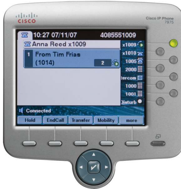
Figure 2. Close-Up of Display and Lighted Line Keys
